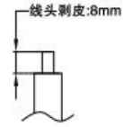
导线规格: 24-10AWG
